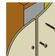
The ring shank nails can be attached with either a nylon hammer or nail gun. For a perfect match to the board material, the nail and screw heads can be provided with a RAL colour coating.
