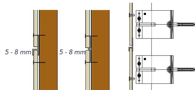
Wooden substructure with closed (left) and semi-closed (right) horizontal joint
