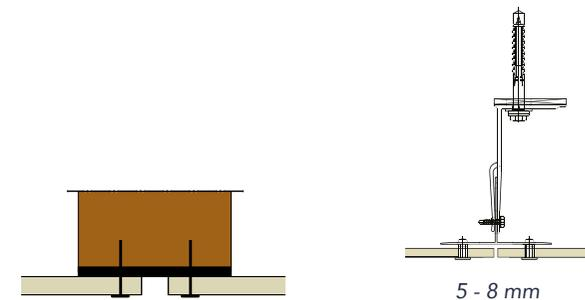
Wooden substructure, vertical joint solution with EPDM foam gasket
