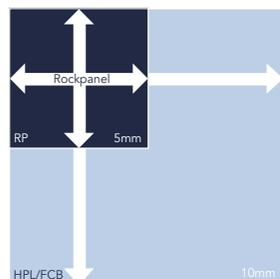
Linear elongation due to temperature fluctuation
