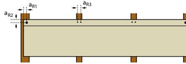
**Maximum permissible building height (m) Lines<sup>2</sup> 10 mm with a 2-field span, fixed using a single Rockpanel ring shank nail, 2,1/2,3 x 27 mm at the intermediate battens.**
