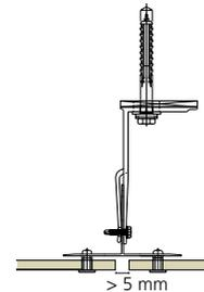
Aluminium substructure, vertical joint solution
